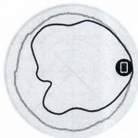
Figure 3 - T310d 5GHz Azimuth Antenna Patterns
